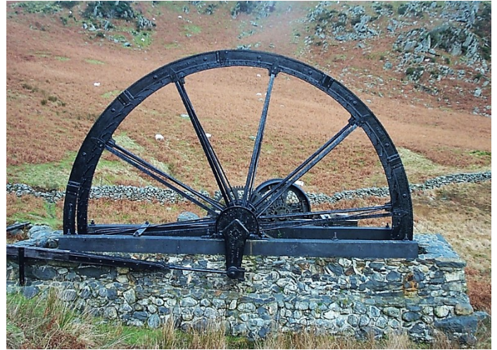
Figure 404: Cwm Ciprwth copper mine site. (left) Rod system connecting the water wheel to an angle bob which operated pump rods in the mine shaft. (right) Water wheel providing power for pumping, and a geared winding drum for raising buckets of ore from the mine shaft.
