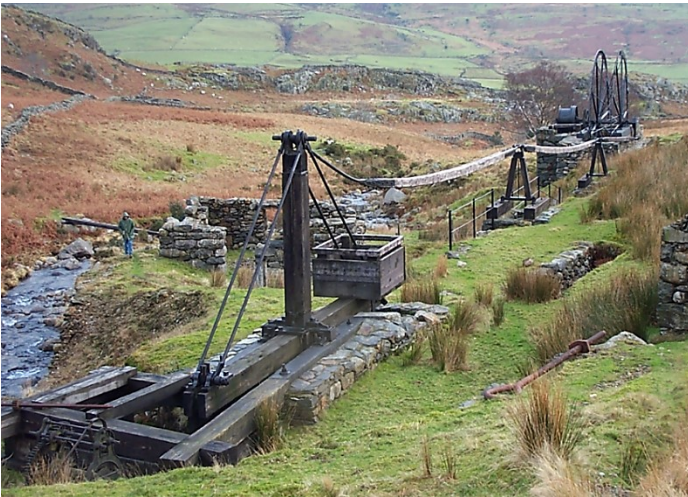
Figure 404: Cwm Ciprwth copper mine site. (left) Rod system connecting the water wheel to an angle bob which operated pump rods in the mine shaft. (right) Water wheel providing power for pumping, and a geared winding drum for raising buckets of ore from the mine shaft.
